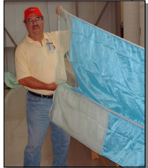
Bert Brown inspects and refolds the panels of a semi-steerable parachute. ( editor's note ... It's my chute. And I have never complained )
